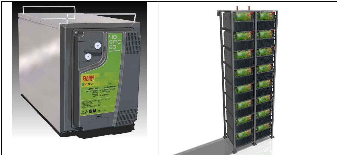
Figure 9 (left) is Fiamm’s Sodium Nickel battery offering. The unit is in a highly insulated stainless steel case to contain the nearly 300 degree (C) operating temperature. The two circles on the upper left are the output connections. The small door at the lower front-left is access to connectors for control and monitoring. The figure to the right is a rack of Sodium Nickel cells delivering 3,200 AH. But hold the sulfur, it doesn’t smell good right now...
