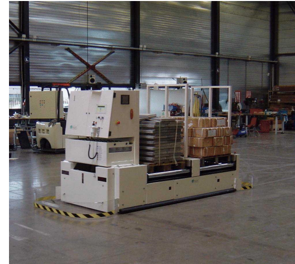
AGV moving material in a manufacturing setting
